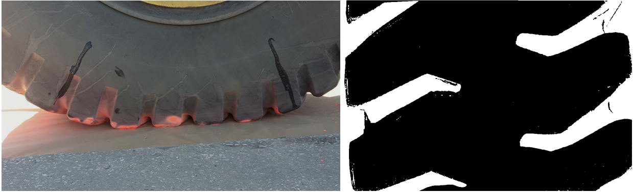
Figure 6.6: Tire foot print taken in the field.
