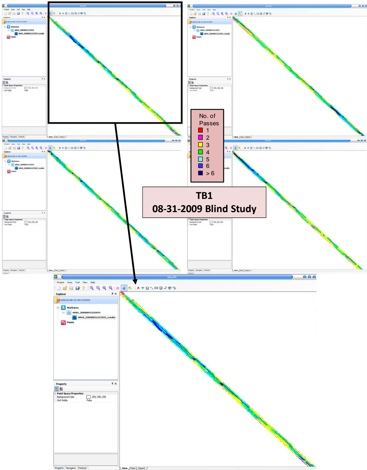
Figure 55. Example pass coverage maps from day 1 blind study – TB1 (approximate mile posts 95 to 97)
