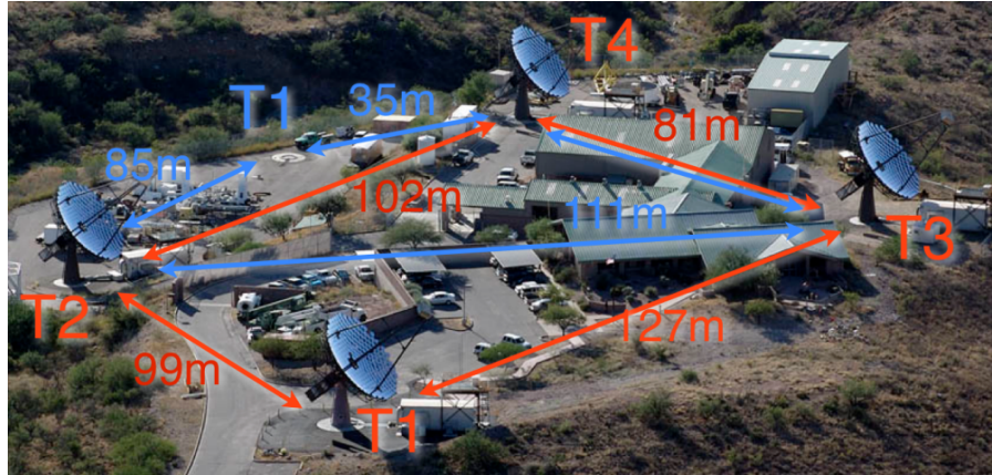
Figure 3.6: Distances between individual telescopes of the VERITAS array. Blue lines identify distances between telescopes in the V4 epoch. Red lines identify distances in the V5 and V6 epochs.
