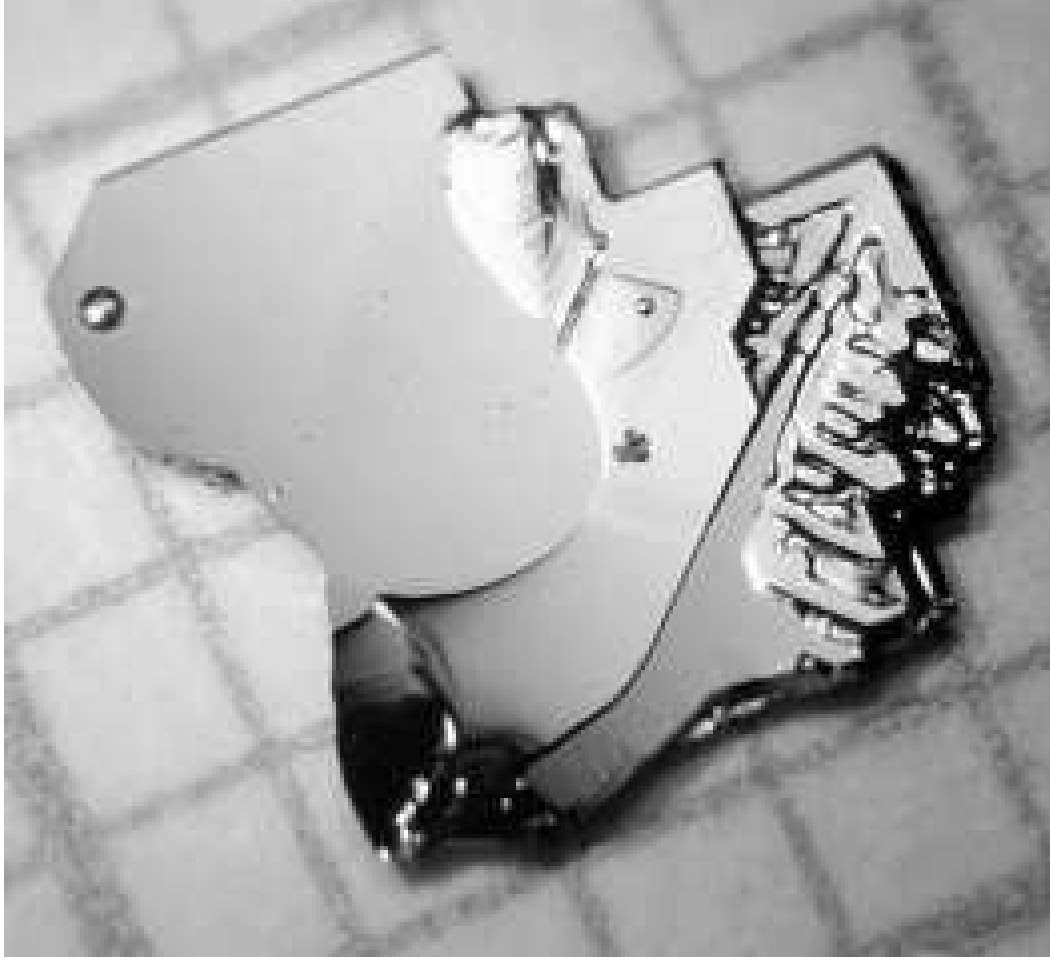
Fig. 1. As-grown single crystal of \text{TbFe}_2\text{Ge}_2 on a millimeter-scale paper. The round droplet on the upper left is solidified Sn flux. Dendritic growth along the [110] directions can be seen on the right side of the crystal.
