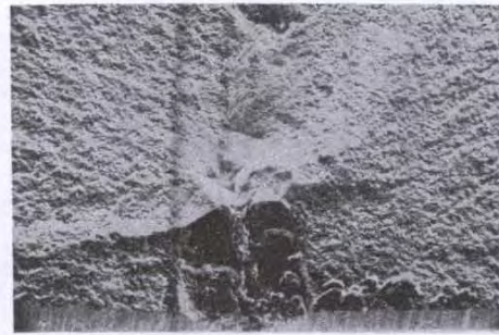
Figure 6. Fracture surfaces of specimen 1-4, showing fracture origin at ultrasonically detected 25 \mu\text{m} (0.001 inch) void.
