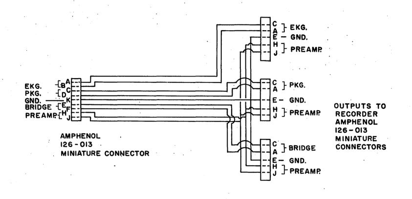
Figure 25. Electronic circuit design of the combined Wheatstone bridgetransistor preamplifier unit for processing and amplifying information from electrocardiographic, phonocardiographic and pneumographic transducers
