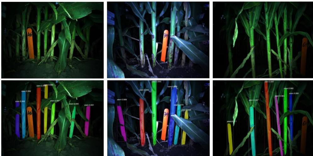
Figure 3.9. Instance segmentation results produced by Mask R-CNN. Examples of the original images are displayed in the top row and their corresponding segmentation results are illustrated in the bottom row. Each color area indicates a segmented stem instance.
