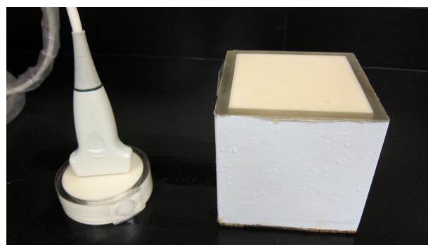
FIG. 1. (Color online) Data collection set-up. The sample was scanned first and the reference was imaged under the same system settings used for the sample.
