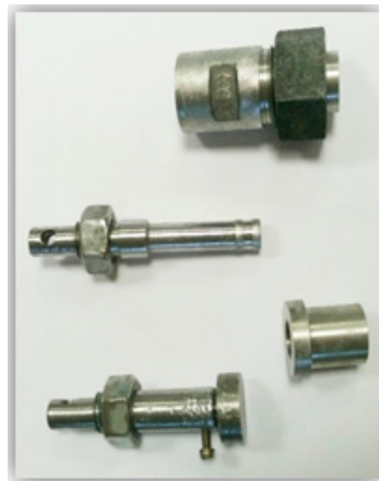
Figure A2. Metal fixtures and sleeves (right) used in the structural modification (pelletization) of carbonized refuse-derived fuel (CRDF).
