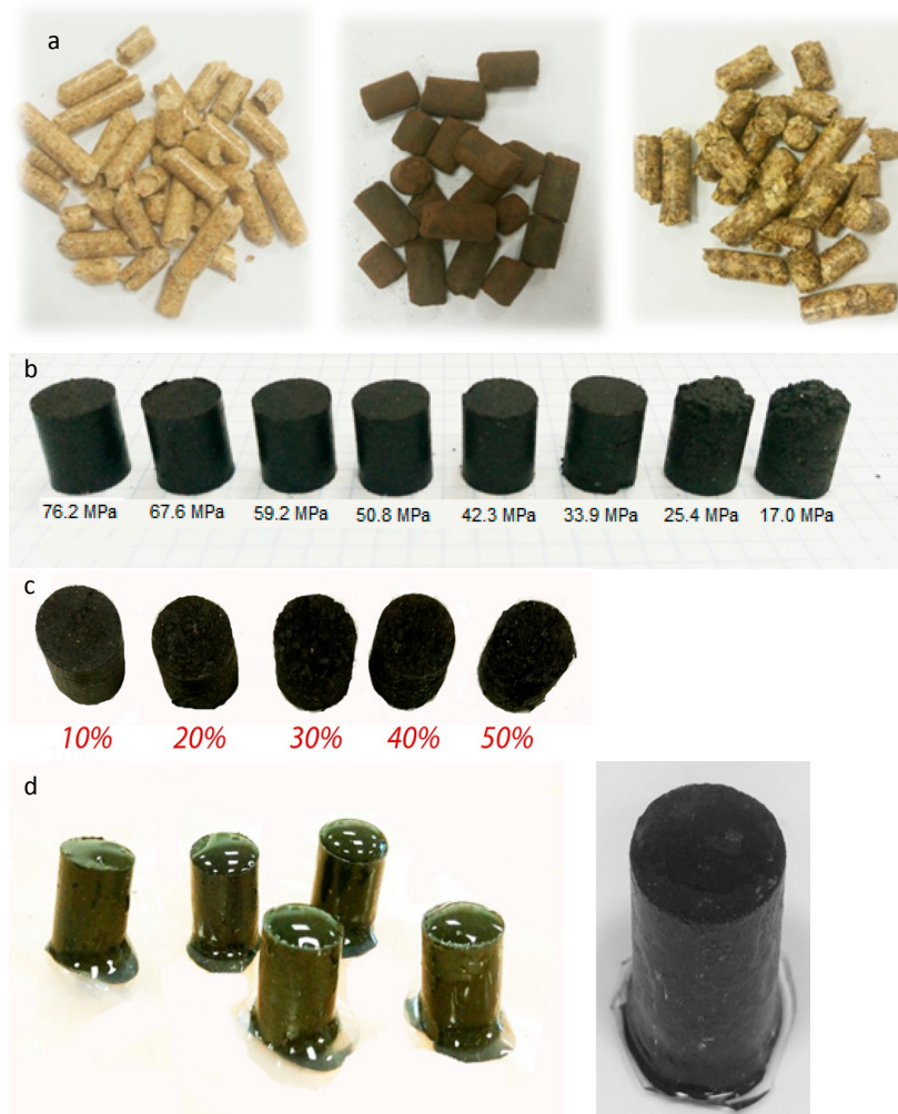
Figure A1. Pellets tested in the experiment: (a) reference pellets from biomass: pine (left), lignocellulosic (middle), from corn husks (right); (b) carbonized refuse-derived fuel (CRDF) pellets produced by applying pressure from 17.0 MPa to 76.2 MPa; (c) CRDF pellets produced with a pressure of 50.8 MPa and a variable proportion of water glass from 10% to 50%; (d) CRDF pellets produced with a pressure of 50.8 MPa impregnated with water glass: left: samples immediately after impregnation, right: sample after drying.
