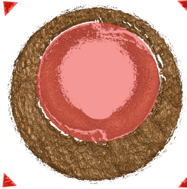
Figure 3.2: Cartridge case scan with highlighted regions to be removed during pre-processing.
