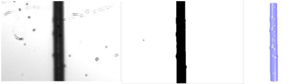
Fig. 12. Micro-filament detection in focused regions of interests
