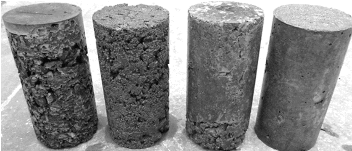
Figure 4. Cylinders made with mixtures with increasing cementitious content from 400 to 700 lb./yd. 3
