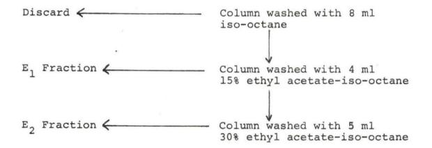
The tubes' contents (the  $E_1$  and  $E_2$  fractions) were evaporated in a 45C water bath. The sides of the tubes were washed down with 1 ml of ethyl acetate and the solvent was completely evaporated.
