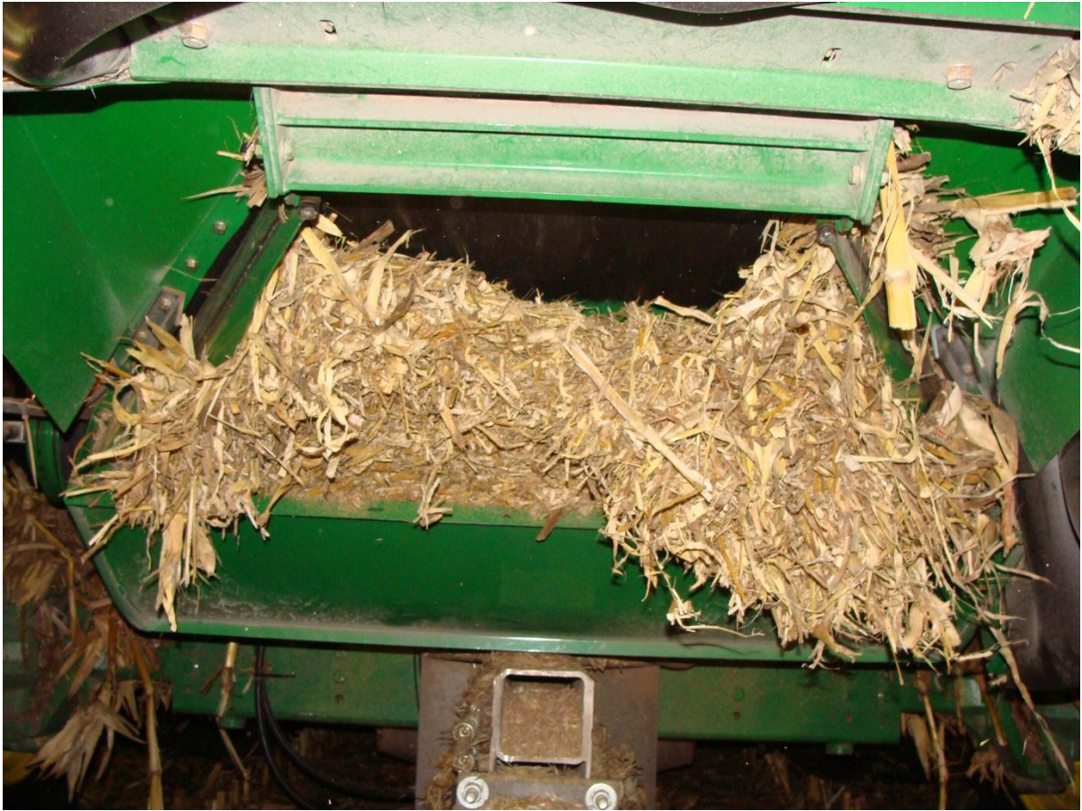
Figure 25: Image illustrating plugging caused by the MOG split vanes at chopper discharge
