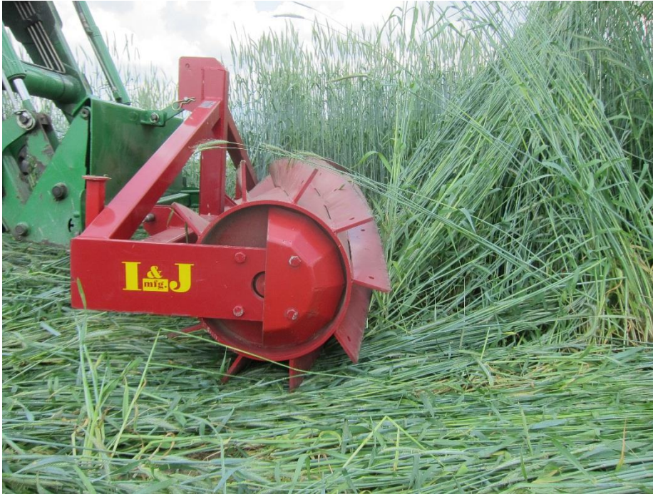
Fig. 1.1. A roller-crimper mounted on a front-end loader rolling a cereal rye cover crop.
