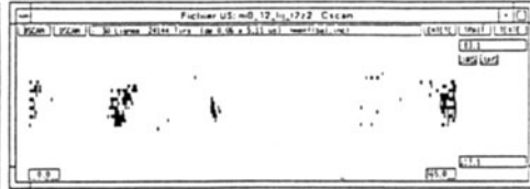
Figure 7. UT CSCAN tube image
