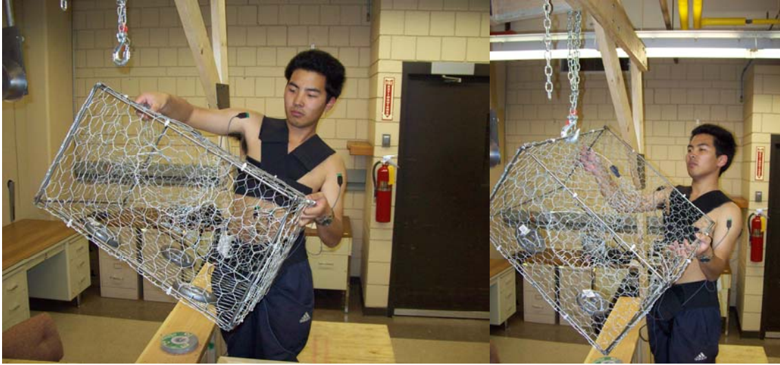
Figure 6. Shake crab pot task (left without hook (no intervention), right with hook support (intervention)).
