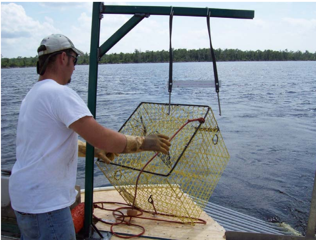
Figure 4. The Crab Pot Boom intervention mounted to the side of the fishing boat.
