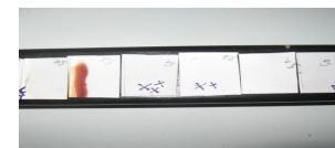
Figure 4. Color and odor identification of 2-acetyl-1-pyrroline after 2,4 dinitrophenyl hydrazine stain and alkali addition
