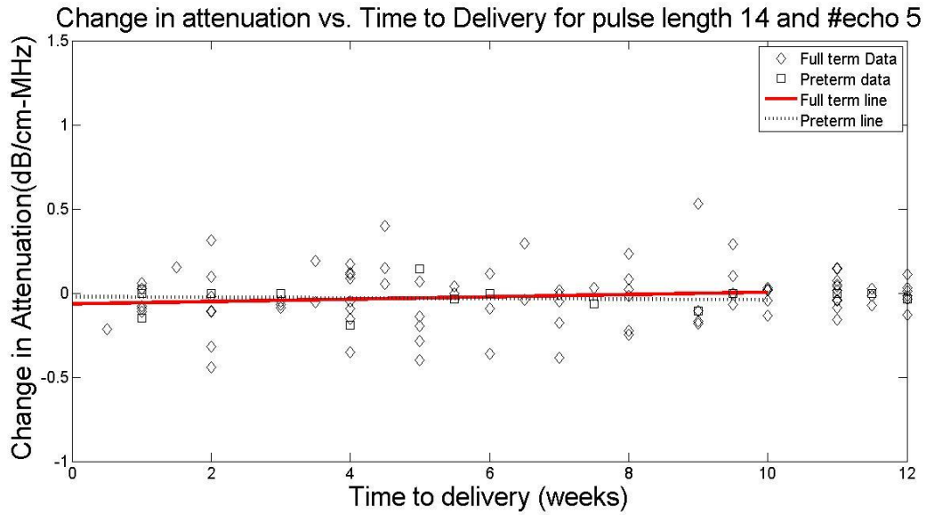
Figure 60: Change in attenuation vs time to delivery for pulse length of 14 and 5 independent echoes
