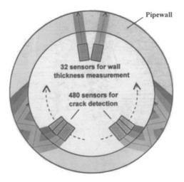
Figure 2. Sensor arrangement for ultrasonic crack inspection (schematic).
