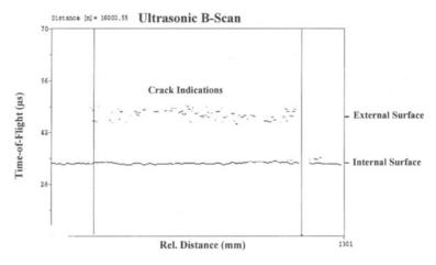
Figure 6. B-scan showing crack indications from part of a SCC colony at the external side of a 56" pipe joint. Here, the crack lengths are below 30 mm, the estimated depths are up to 3 mm.
