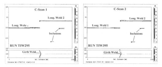
Figure 3. Comparison of C-scans from the same pipe joint recorded during two separate runs (26" crude oil pipeline). The C-scans at the bottom show the results of the wall thickness sensors indicating the location of the girth weld.
