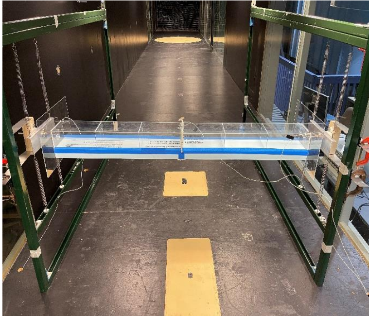
Figure 3.1 Test section interior with suspended section model
