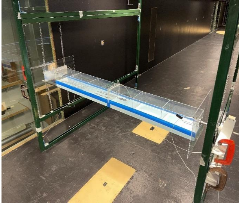
Figure 3.2 Suspension System used for the section model tests
