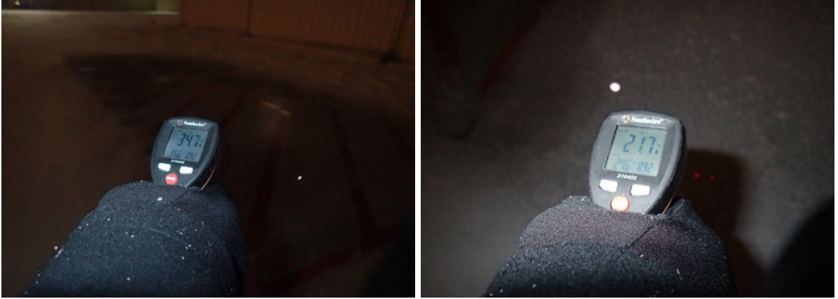
(a) (b) Figure 21 Surface temperature: (a) ECON surface temperature during Operation time and (b) adjacent PCC Slab
