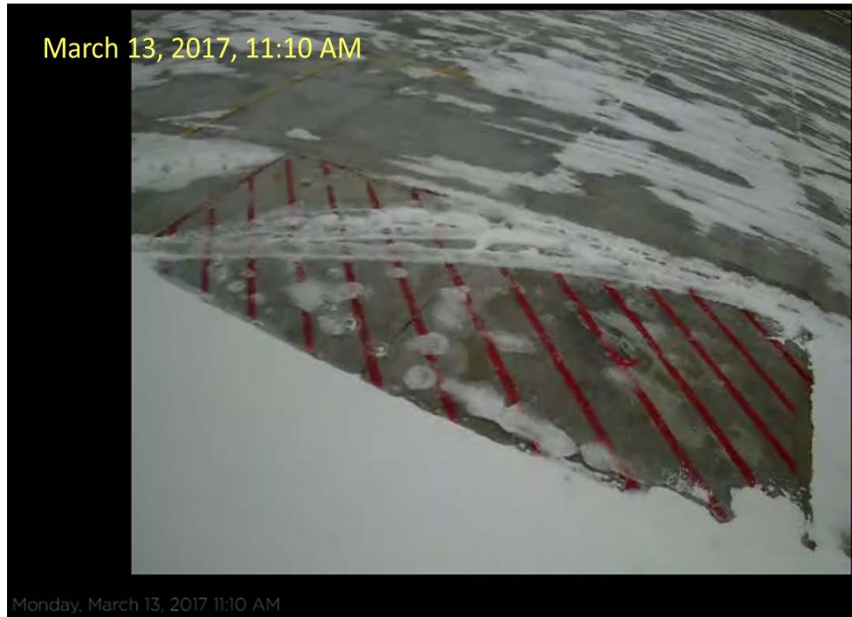
Figure 28 Performance of the ECON HPS at DSM, IA: (a) before turning on the HPS (b) after 1 hours and 5 minutes of operation, (c) after 1 hours and 23 minutes of operation, (d) after 1hours and 50 minutes of operation
