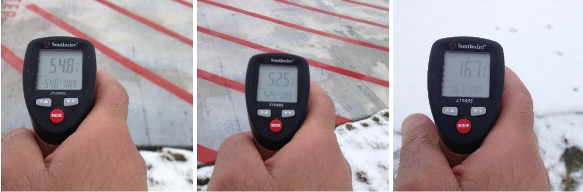
Figure 8 Surface temperature reading at ECON slab 1 and adjacent slab during operation time
