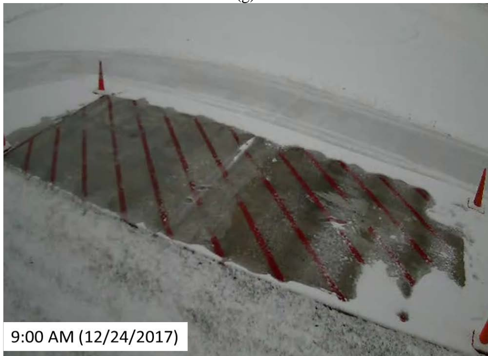
Figure 30 Performance of the ECON HPS at DSM: (a) system turned on at 3:30 AM (b) after 1 hours of operation, (c) after 2 hours of operation, (d) after 4 hours operation, (e) after 4 hours and 55 minutes operation, (f) after 4 hours and 56 minutes of operation, (g) after 5 hours and 10 minutes of operation, and (h) after 5 hours and 20 minutes of operation
