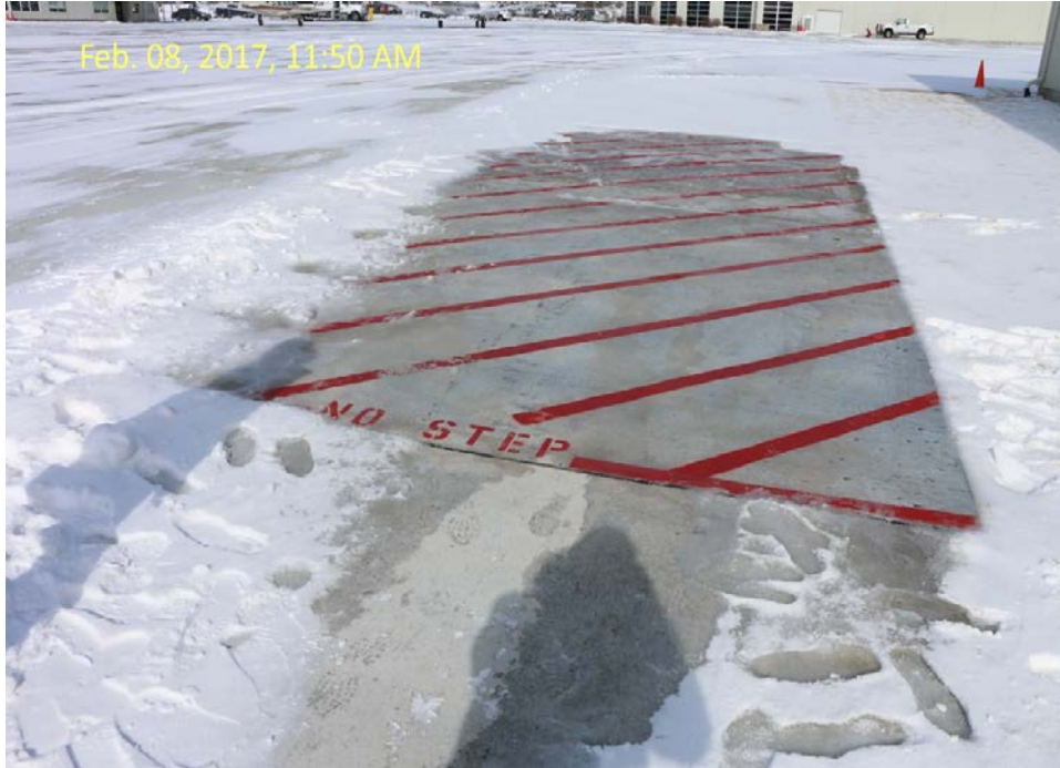
Figure 25 Performance of the ECON HPS at DSM, IA: (a) after 2 hours and 48 minutes of operation, (b) after 3 hours and 45 minutes of operation, (c) after 4 hours and 12 minutes of operation, and after 4 hours and 38 minutes of operation.
