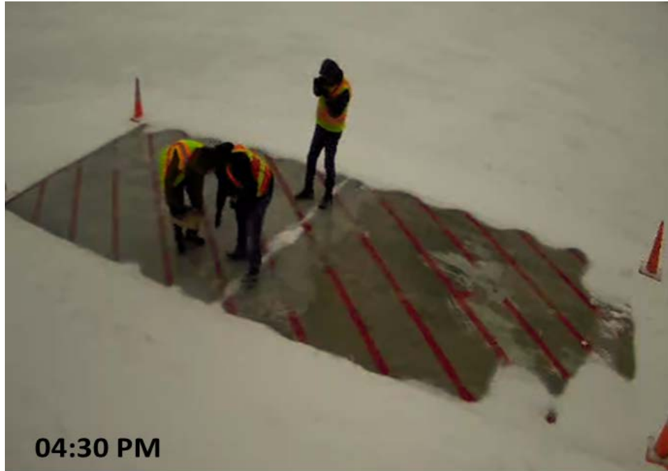
Figure 36 Performance of the ECON HPS at DSM: (a) system turned on at 12:10 PM (b) after 2 hours of operation, (c) after 3 hours of operation, and (d) after 4 hours and 20 minutes of operation
