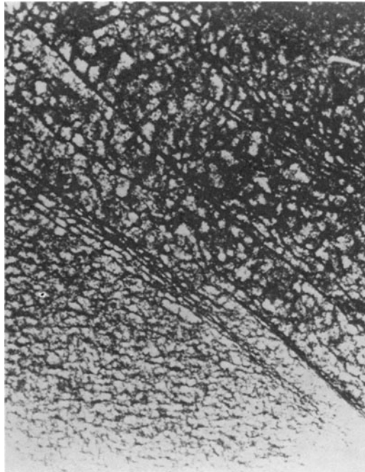
Figure 6: a.) X-ray topograph (XRT) of a section of LEC-grown GaAs crystal showing a dense network of dislocations.
