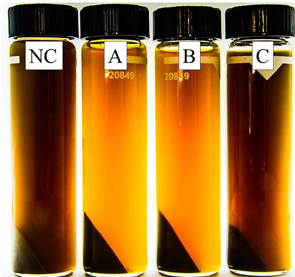
Figure 2. Oral fluid specimens following treatment. NC = negative control; A = formulation A (chitosan 100 ppm, Tween-20® 0.1%, BSA 0.5%, xylene cyanol 1 ppm); B = formulation B (chitosan 100 ppm, BSA 0.5%, xylene cyanol 1 ppm); C = formulation C (Tween-20® 0.1%, BSA 0.5%, xylene cyanol 1 ppm)
