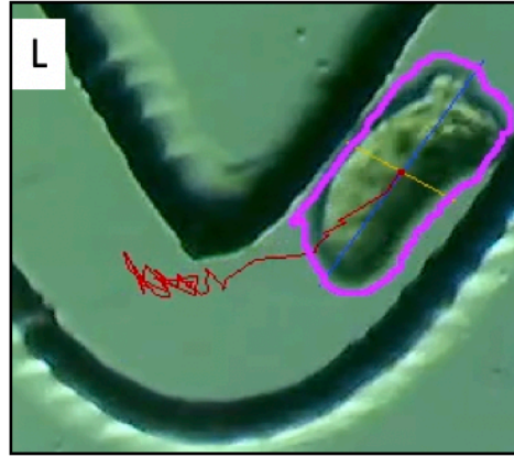
Figure number 2.4 JKL : Centroid distance and track distance are the two parameters used to express the movement and migration of the somules as they travel through the sinusoidal channels of the microfluidic chip. J. Tracing S. mansoni somule as it travels through the sinusoidal channel of the microfluidic chip. K. The parameter used for the expressing the movement of the somule at a single point is centroid distance, denoted by red . In the somule. the major axis is denoted by blue and minor axis is denoted by yellow. The shape of the somule is denoted by pink. L. The parameter used for the expressing the migration of the somule from one point to another track distance, denoted by red. In the somule. the major axis is denoted by blue and minor axis is denoted by yellow. The shape of the somule is denoted by pink. The software was designed by Dr. Zach Njus and Dr. Santosh Pandey.
