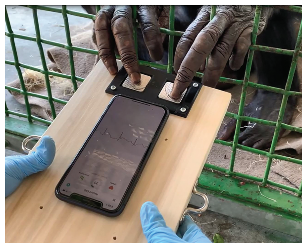
Figure 1 —Photograph demonstrating the KardiaMobile device mounted to a wooden block and used during a training session with a male bonobo. As shown in the photo, a sterile lubricant was applied to the device sensors to increase conductivity. The ECG tracing is visible on the smartphone shown in this image. Completed ECG tracings were saved as PDFs and submitted to evaluators for review.
