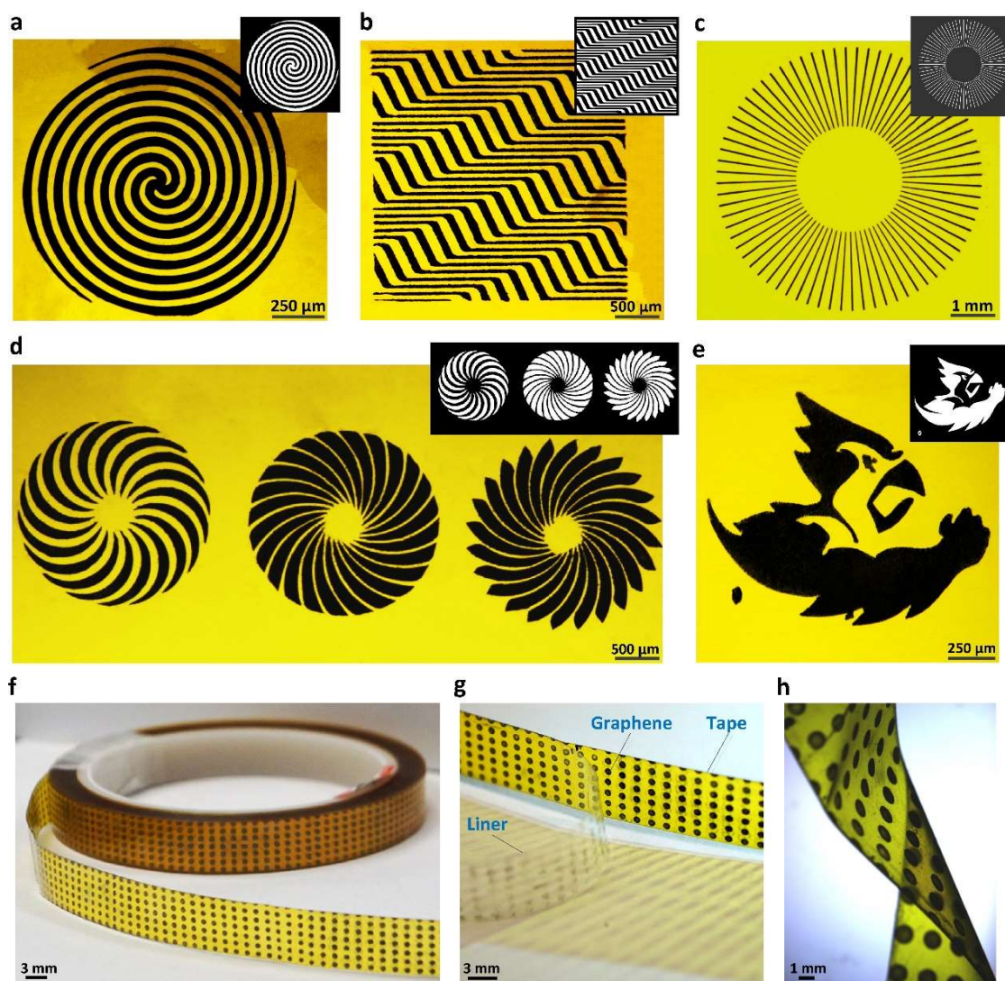
Figure 2.2 (a)–(e) Versatile graphene patterns formed on the polyimide tape using the proposed method. (f)–(h) Formation of graphene patterns on the relatively large polyimide tape roll with liner. The transferred graphene patterns are protected by a non-sticky liner.
