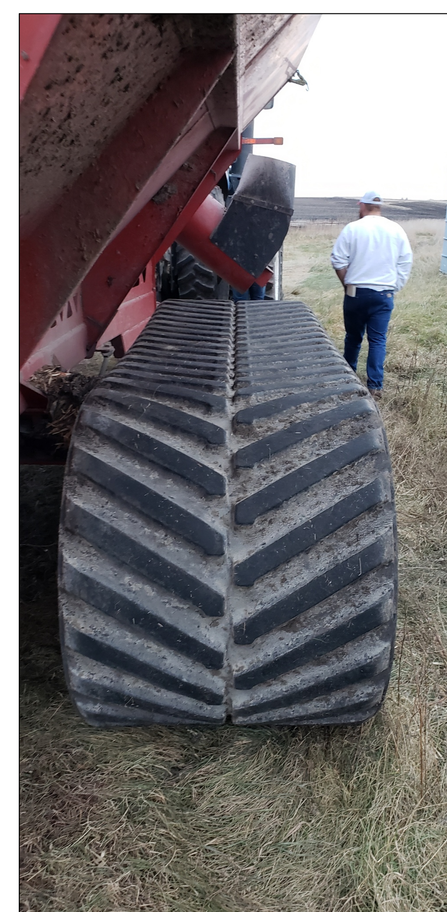
Tracks on grain carts are popular to help decrease compaction level by spreading out the weight.
