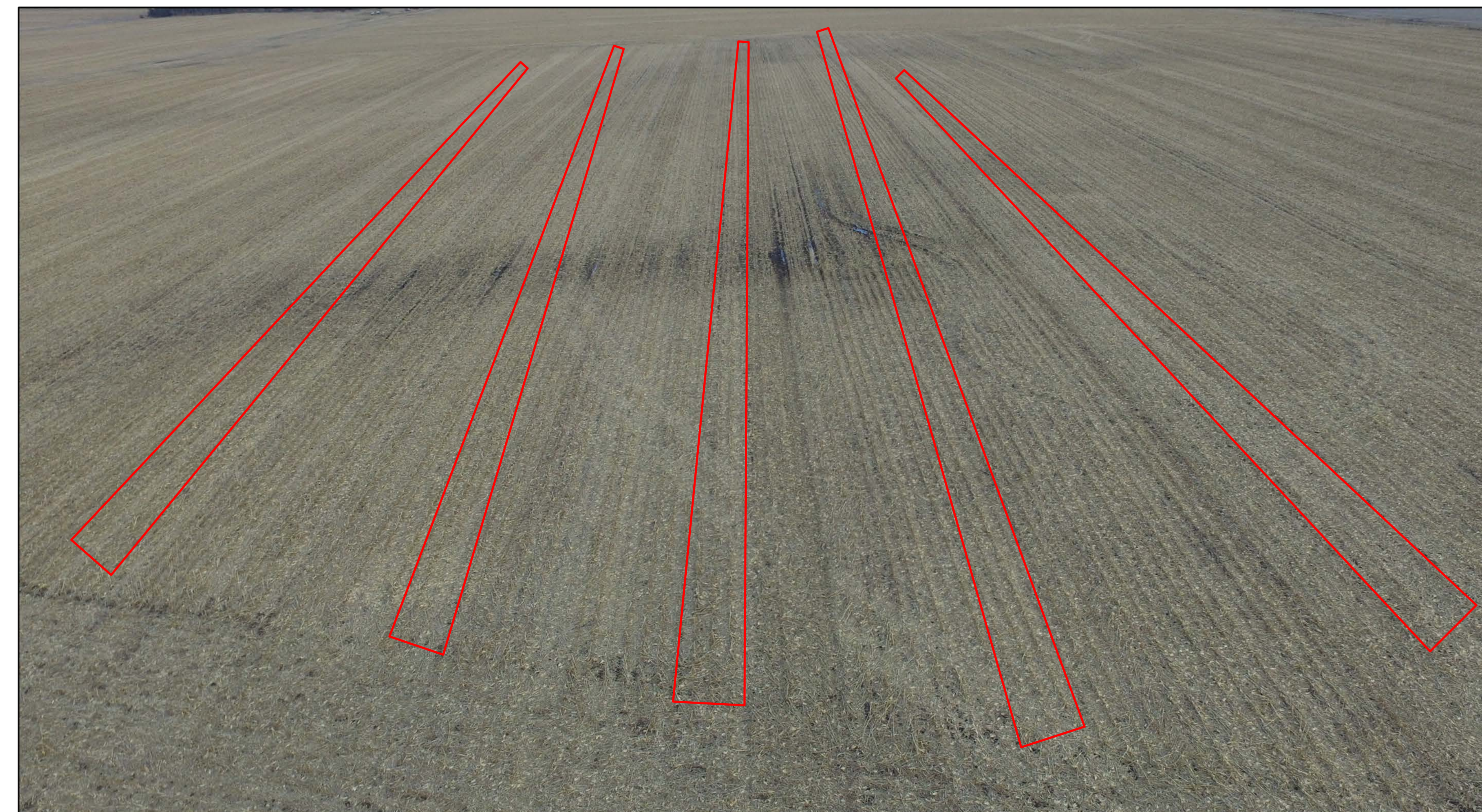
Drone footage of field where red outlined areas represent grain cart path. Inside outline, soil pressure averaged 75 PSI. Outside grain cart path, average compaction level was 25 PSI.
