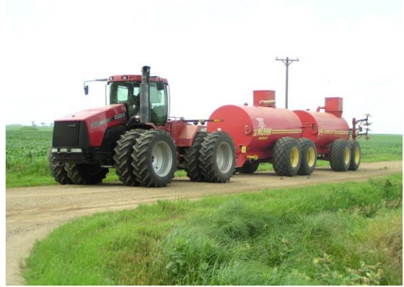
(b) Tractor with two liquid manure applicator tank
