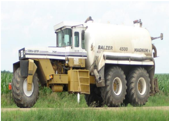
(c) Terragator with single wheel front axle
