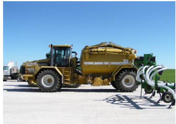
(d) Terragator with two wheel front axle
