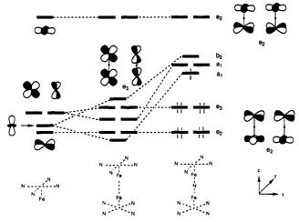
Figure 4. The building up of the orbitals of  $[(NH_2^-)_4FeNFe(NH_2^-)_4]^{4-.45}$ From left to right: the orbitals of the pyramidal N<sub>4</sub>Fe in which Fe is displaced by 0.32 Å out of the N<sub>4</sub> plane; two such pyramidal N<sub>4</sub>Fe units brought to 3.322 Å separation between the irons; the orbitals of the composite nitrido complex. The electron count shown is that appropriate to a low-spin Fe-N-Fe complex.
