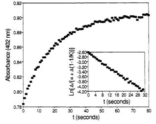
**Figure 1.** Representative absorption (402 nm) vs time plot for eq 9 at 20 °C.  $[N \equiv Mn(TTP)]_0 = 5.49 \times 10^{-6} \text{ M}$ , and  $[Mn(OEP)]_0 = 4.83 \times 10^{-6} \text{ M}$ . The inset shows a plot of  $\ln \{\Delta / [\alpha + \Delta(1 - K^{-1})]\}$  vs t.
