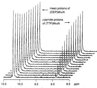
Figure 2. Stacked plot from <sup>1</sup>H NMR kinetics run at 40 °C showing spectra recorded at 20-min intervals.  $[(OEP)Mn \equiv N]_0 = 3.94 \times 10^{-3}$  M, and  $[(TTP)MnCl]_0 = 1.01 \times 10^{-3}$  M.
