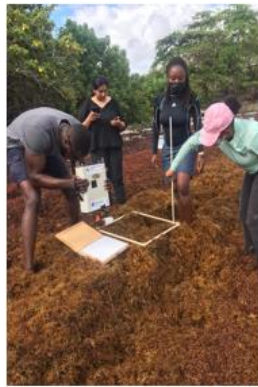
Field spectrometer (SVC HR-1024i) data collection Method 1 (Barbados)
