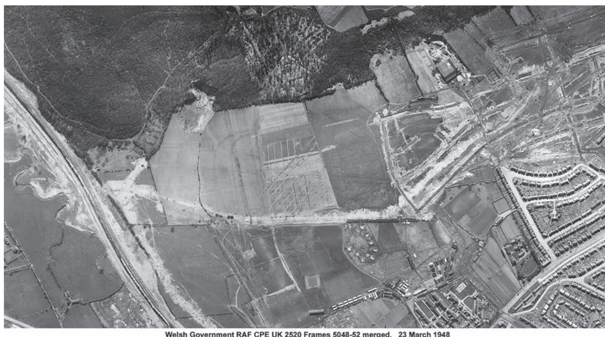
Fig. 3. Vertical aerial photo of Trelai Park in 1948 showing network of recently installed land drains. Crown copyright Welsh Government
