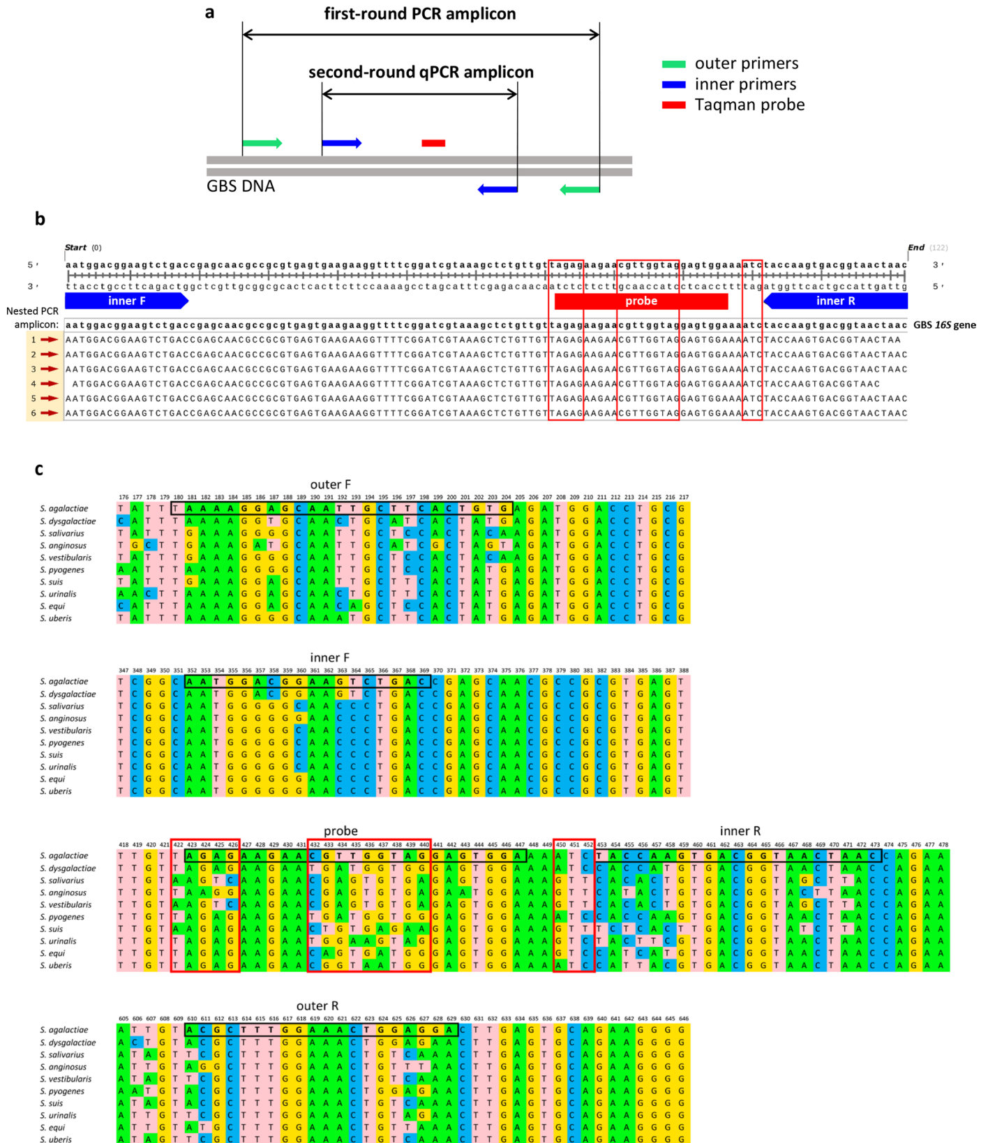
Extended Data Fig. 2 | Nested PCR-qPCR assay to detect the 16S GBS gene.
