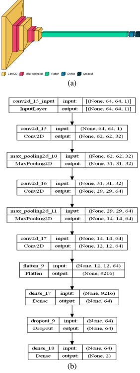
FIGURE 4. The structure of the proposed imgCNN Model
