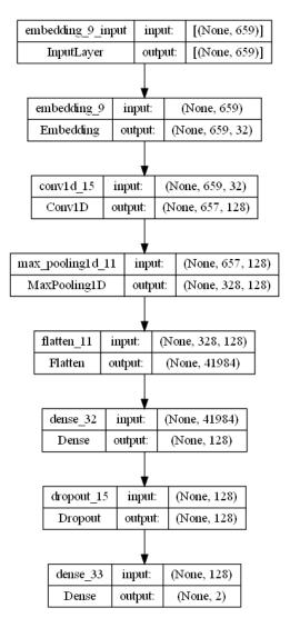
FIGURE 5. The structure of the proposed txtCNN Model
