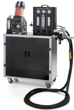
Fig. 2. HVOF spray equipment
