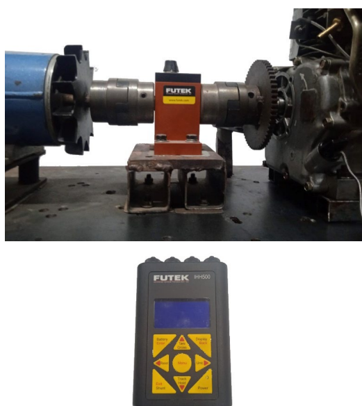
Fig. 10. Futek TRS705 torque sensor assembly and specifications
