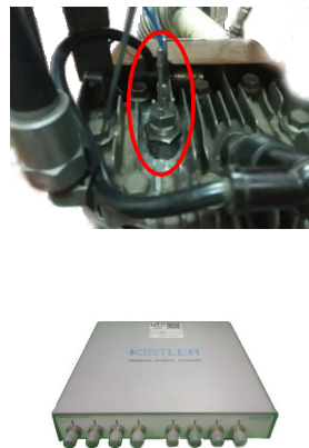
Fig. 8. In-cylinder pressure sensor, conditioning, and assembly
