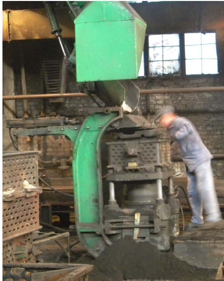
Fig. 16. Production of top half-forms by additional pressing without rotating the half-forms
