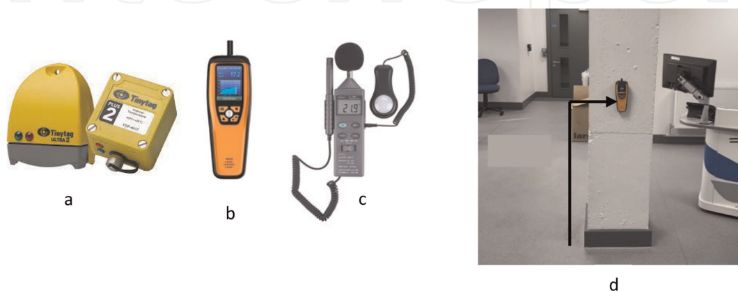
Figure 3. Showing the equipment used and typical Temtop equipment placement in the classroom.
