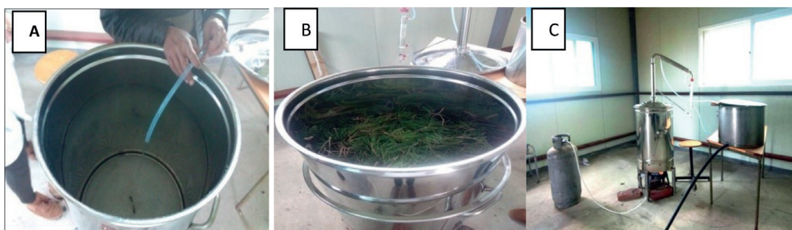
Figure 1. Extraction of essential oils from Pinus halepensis needles by steam distillation. A: Water filling up to separation grid level; B: Introduction of plant material in the alembic. C: Complete assembly.
