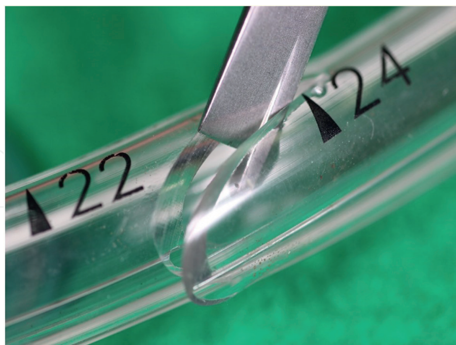
Figure 2. The cause of tube rupture was damaged by a bone chisel used during maxillary bone dissection.
