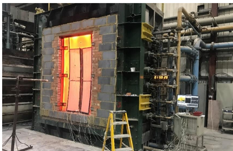
Figure 2 Furnace Fire Testing
