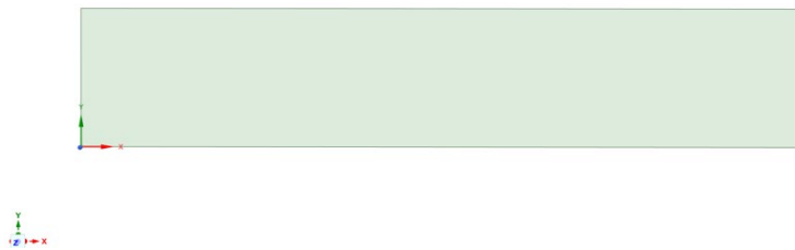
Fig. 62 Geometry of the single layer jute/PLA tensile test specimen in ANSYS.
