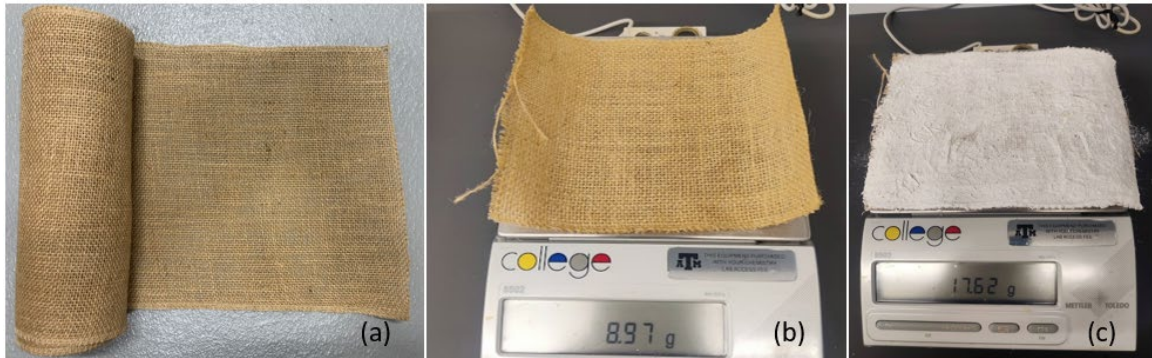
Fig. 49(a) Woven jute fiber used in this research, (b) weighted single layer jute fiber, and (c) weighted PLA coated jute fiber.
