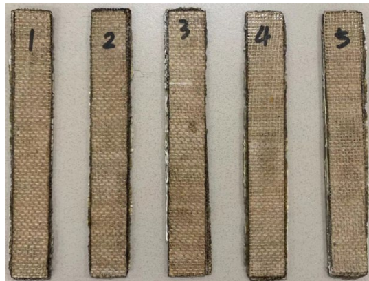
Fig. 53 LOM printed PLA infused woven jute fiber reinforced biocomposites [110].
