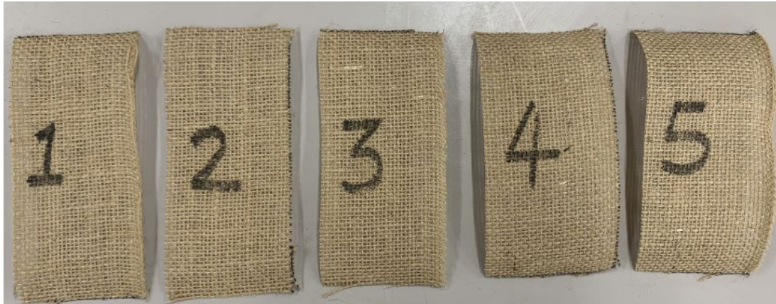
Fig. 56 Woven jute fibers cut for tensile tests following ASTM D5035 – 06 [110].
