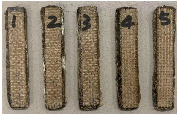
Fig. 58 LOM prototype printed flexural test specimens [110].
