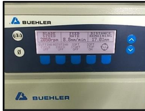
Figure (7): Operating parameter of the diamond saw machine. (Isomet 4000).
