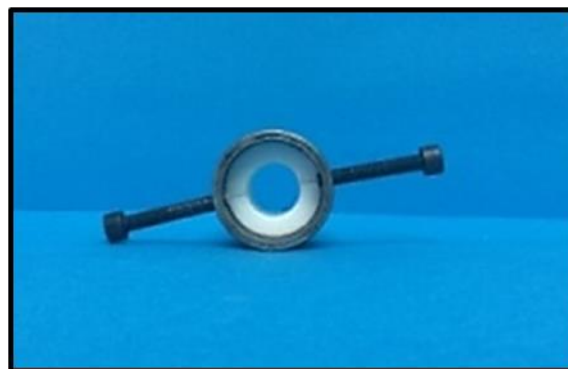
Figure 1 (Top view) shows a teflon mold with a corresponding metal ring and parallel screws.
