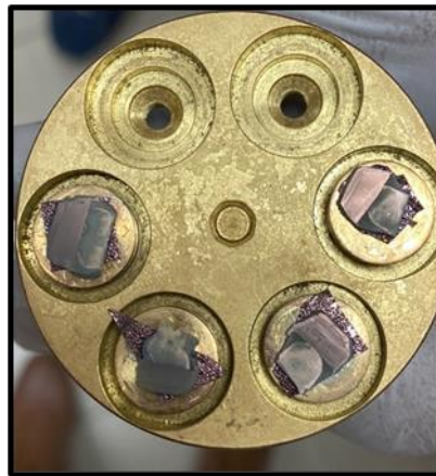
Figure (16): Slices after gold coating.
