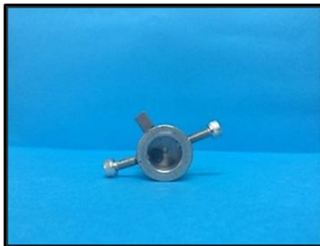
Figure (5): L-Shaped gripping attachment (Front view) with perpendicular axial grooves (arrows).
