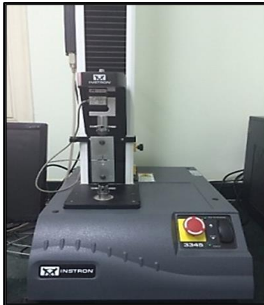
Figure (11): Jig mounted on the Universal testing machine.
