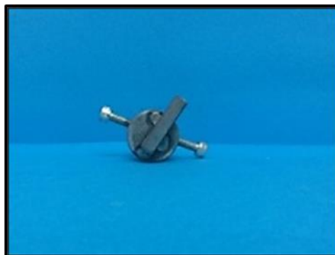
Figure (6): L-Shaped gripping attachment (Rear view) - Perpendicular metal rod (arrow).
