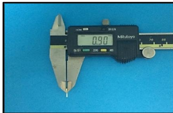
Figure (9): Measuring the beam's thickness at the composite-dentine interface.
