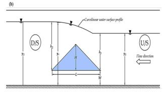
Figure 2. Triangle side orifice (a) 3D view, and (b) water surface profile view.
