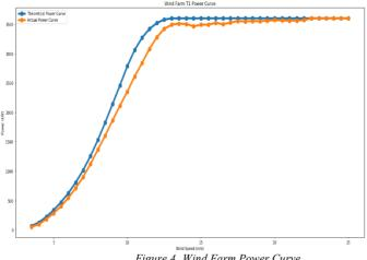
Figure 4. Wind Farm Power Curve
