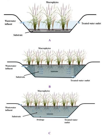
Figure 4. Constructed wetlands types A: free water surface, B: horizontal flow subsurface, and the vertical subsurface flow.
