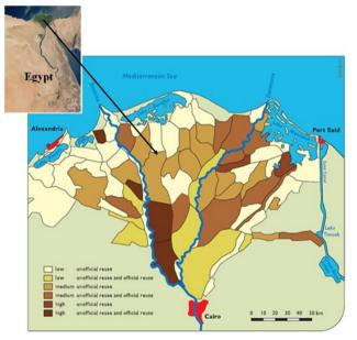
Figure 7. Reuse drainage water in Egypt's Delta.
