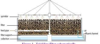
Figure 1. Trickling filter schematically.
