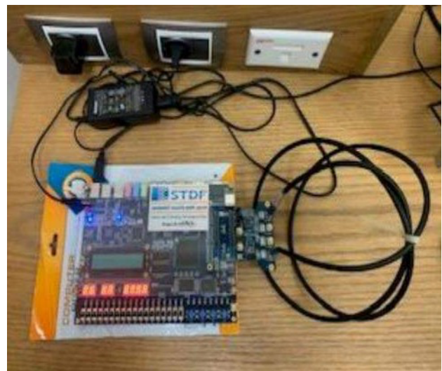
Figure 7: Experimental setup for the Altera DE2-70 board, with the A/D converter card
