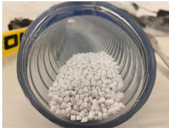
Figure 3. Particle accumulation consisting of 2032 PET-particles in a flexible PVC pipe. The particles are cylindrical with a length of 2.8 \pm 0.1\text{mm} and a diameter of 2.3 \pm 0.3\text{mm} , and have a density of 1395 \pm 3.3 \text{ kg/m}^3 .
