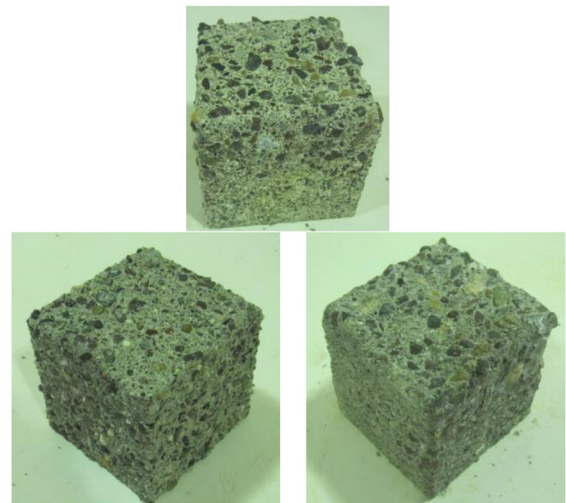
Fig. 12 Concrete sample after being exposed to the acid environment
