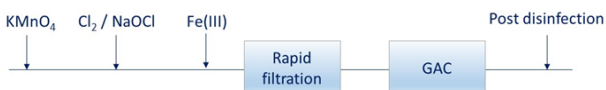
Fig. 3 Typical breakpoint chlorination treatment combined with iron, manganese and arsenic removal (breakpoint chlorine dose is applied at the beginning of the treatment process)
